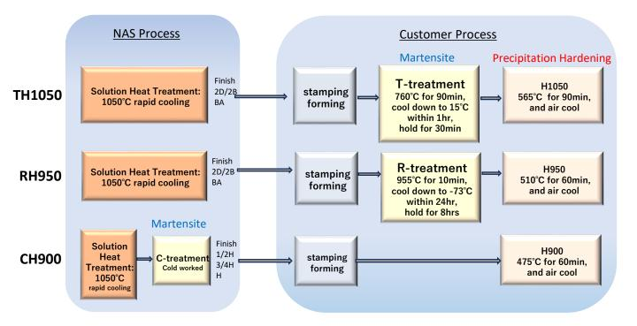
First, the material is changed into a martensitic structure by one of the following methods:
